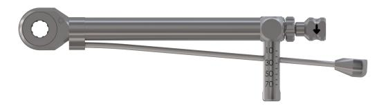
For prosthetic components that require a torque value which ends in a unit of 5 (example 25), the teardrop lever arm should be located between the 20 Ncm and 30 Ncm marks on the shaft as shown above.
